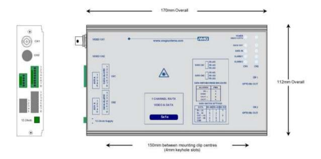
The **AMG5714A9-DIN** is a DIN Rail mountable standalone one channel video receive unit designed to receive 1 video signal and transmit & receive 1 data signal, 1 Bi-directional alarm and 1 Bi-directional audio channel over one Singlemode optical fibre.
